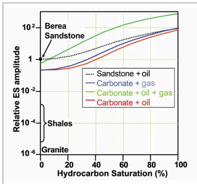
Figure 10. Calculated ES amplitudes (relative to the amplitude for water-saturated Berea sandstone) versus hydrocarbon saturation. HC saturation alters the amplitudes by a factor of 100 or more. The saturation-dependence is large in rock containing some gas. Impermeable rock has low electrokinetic coupling.
