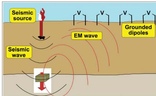
Figure 1. Schematic of seismoelectric (SE) conversion. The seismic wave, generated at the surface, creates a pressure gradient at a rock interface where distorted dipolar structures on pore surfaces produce an electric field. The time-varying electric field propagates to the surface where grounded dipole electrodes detect its arrival.
