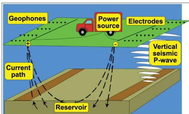
Figure 2. Schematic of electroseismic (ES) conversion. An electric field applied to the electrodes drives current to the reservoir where the largest vertical current converts to the largest, vertically propagating P-wave. Digital accelerometers detect its arrival.
