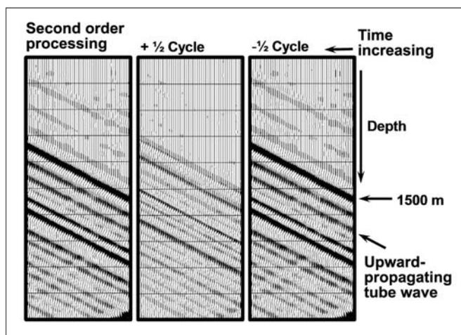
**Figure 9.** Well data showing rectification of the ES signal from west Texas. The data are upward propagating tube wave data from reservoirs below 1500 m deep. The positive and negative portions of the ES wavelets have different amplitudes, as expected for a rectified signal.
