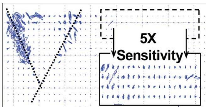
**Figure 4.** Hodogram of horizontal digital accelerometer components at the west Texas site. Surface waves, generated where the electrode crosses a buried pipe, caused the high-amplitude events on the left. The expanded sensitivity on the right shows that the electrodes themselves generate electroseismic coupling. The data are nonlinear ES conversions. The electrode is located along the top of the display.
