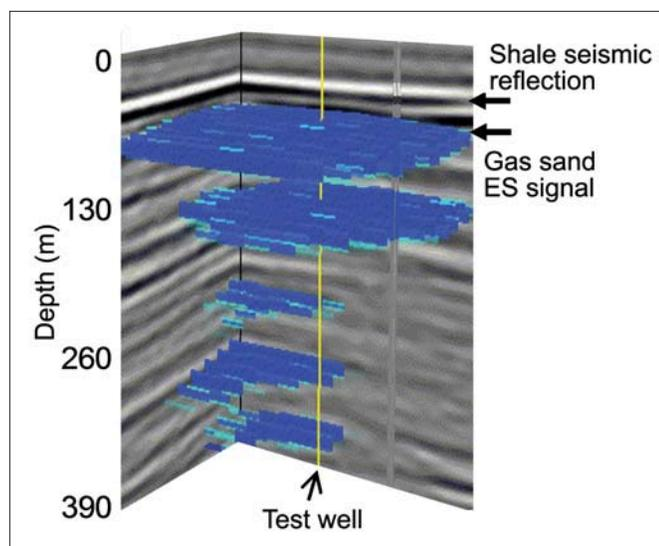
**Figure 7.** ES gas-sand data from the Gulf coast. The background is two sections of a 3D seismic survey. The blue regions are the areas of highest ES amplitude. Low amplitude ES signals are transparent. The shapes and depths of the ES signals are the ones expected for the applied electric fields at the known gas sand depths. A test well, as indicated, confirmed the location of the gas sands.
