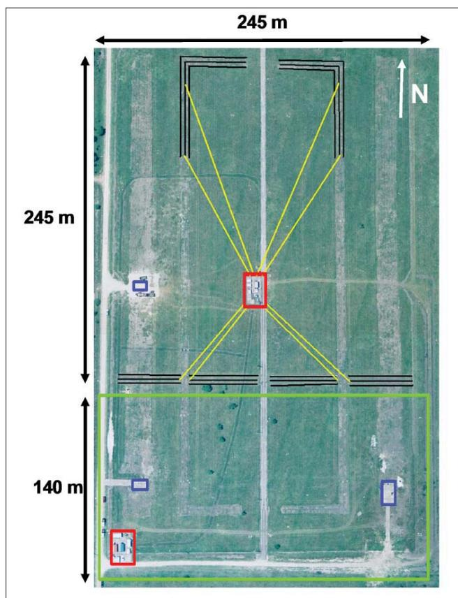
Figure 3. Aerial photo of a Gulf of Mexico coastal site in Texas. The blue boxes are well locations, the yellow lines are bus wires, the black lines are electrodes, the red box in the lower left is the doghouse site, and the red box in the center is the location of the power source. The green box outlines the geophone array of  $10 \times 18$  stations.
