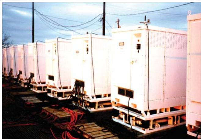
**Figure 6.** PWS field installation in west Texas. Each PWS weighs 3000 kg and produces 350 kW of coded-waveform power at 120 V. They are truck transportable and rest on vibration-isolation skids. The wires from each PWS are 4/0 welder's cable connected to the electrodes.
