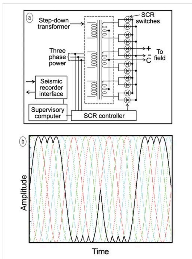
**Figure 5.** The top figure is a block diagram of a power waveform synthesizer or PWS, which combines portions of a three-phase power line to form a specified waveform. The bottom figure illustrates a coded waveform where each of the three phases can have one of two polarities. The black curve is the envelope of selected portions of phases in the waveform.
